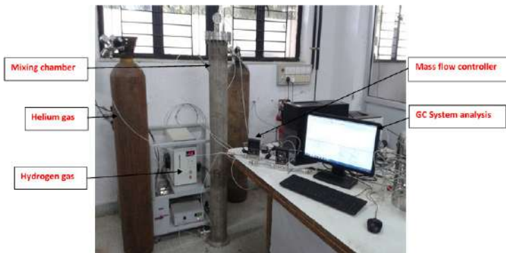
Figure A.2.25. Developed experimental setup for helium purge gas preparation in operation
