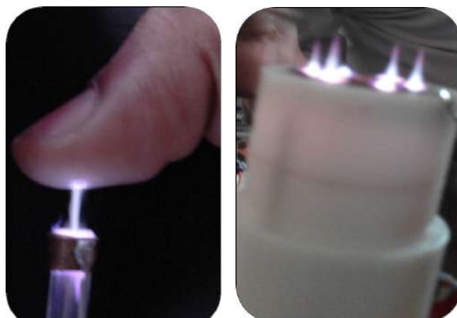
Figure B.1.7 Photo of single jet and multiple jet using atmospheric pressure plasma
