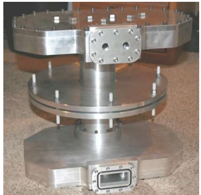
Figure A.3.4.4 The fully assembled mode converter (a) and two mode converters assembled and connected back to back (b) to perform S 11 and S 12 measurements.
