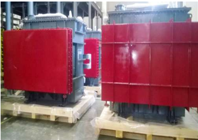
Figure B.2.14 2.8MVA Oil filled multisecondary transformers to IEC standards were manufactured by M/s. T&R (I) Ltd. Ahmedabad.
