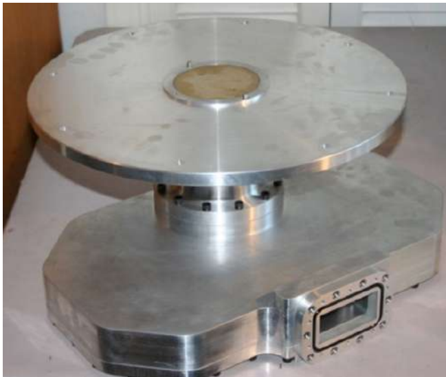
Figure A.3.4.4 The fully assembled mode converter (a) and two mode converters assembled and connected back to back (b) to perform S 11 and S 12 measurements.
