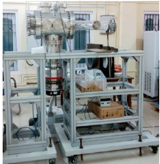
Figure B.3.2 HeliPS setup with glass chamber, expansion chamber, Vacuum pumping system and various gauges.
