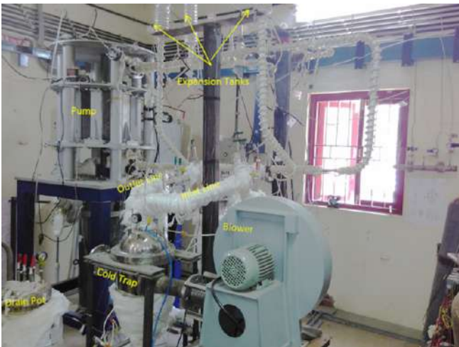
Figure A.2.9. Pb - Li Purification Loop set up with Cold Trap
