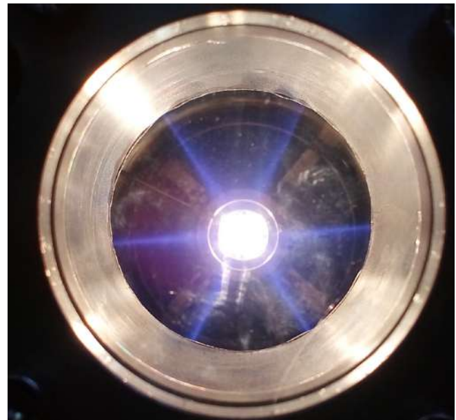
Figure A. 3.10.1 Argon plasma in a profiled multi-cusp magnetic field.
