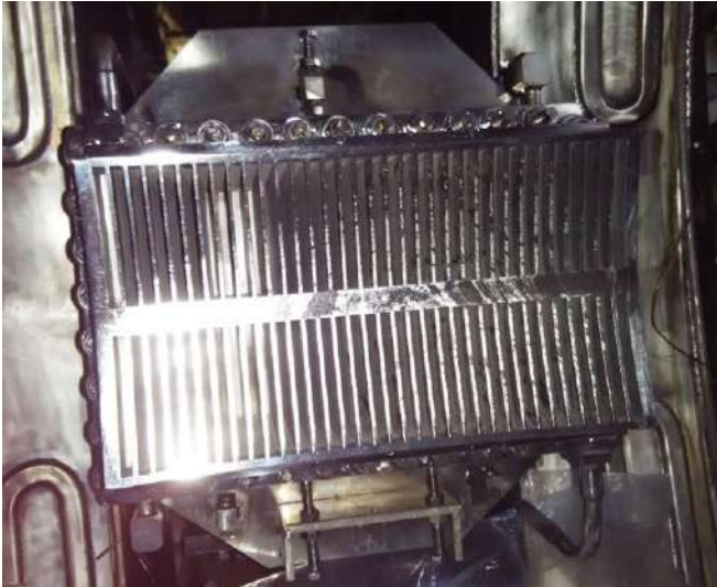
Figure A.1.2.3.1 Stainless Steel Grill Antenna for LHCD launching in SST-1
