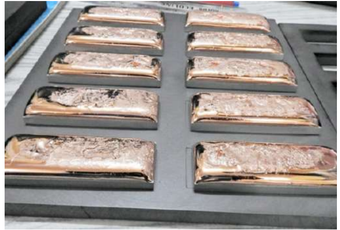
Figure A.2.5 Copper casting on Pure Tungsten Tiles done using Vacuum Brazing Furnace Cu to Cu brazing for FCIPT, Brazing of SS tube to Cu block of Limiter of SST-1 and ongoing brazing and casting activities of DFD group where tungsten and graphite are being brazed to CuCrZr.
