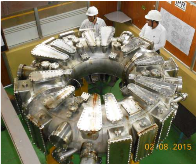
Figure A.1.1.3. Circular cross-section vacuum vessel in the test stand at the institute
