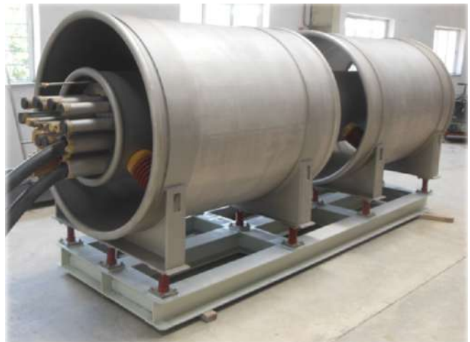
Figure B.2.15 Prototype section of 3.5m of High Voltage Transmission line
