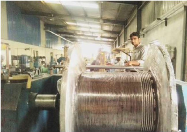
Figure A.2.1 Nb 3 Sn cabling for SST-1 superconducting Central Solenoid
