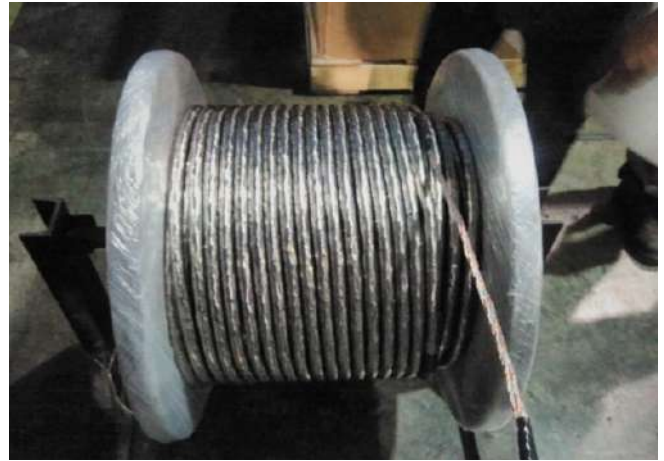
Figure A.2.1 Nb 3 Sn cabling for SST-1 superconducting Central Solenoid
