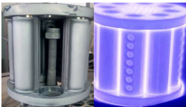
Figure B.1.6 a) Cathodic cage made of hollow tubes with sample in the center b) plasma formed on the cathodic cage.
