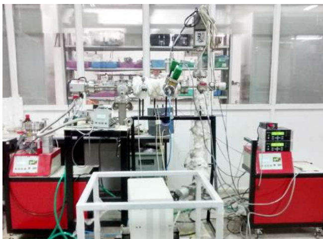
Figure A.2.28 Testing set up for isotope sensor in gas phase
