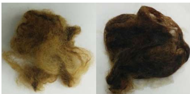
Figure B.1.10 (a) Untreated Merino wool fiber (b) Plasma treated Merino wool fiber
