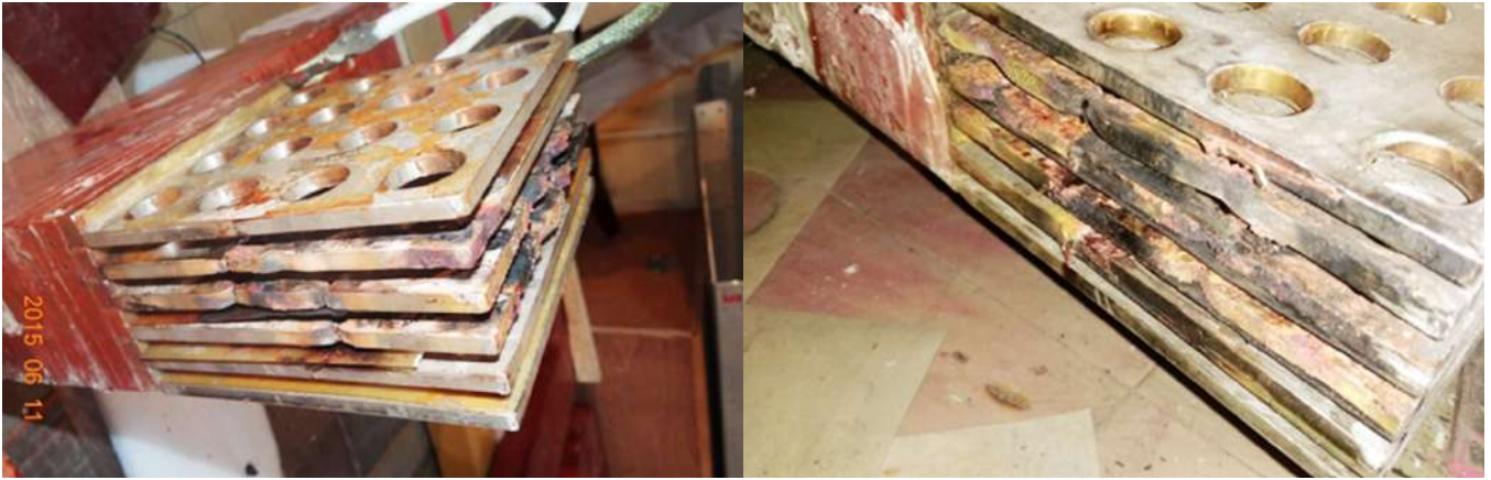
Figure A.1.1.2. The photographs of damaged finger joints of Toroidal magnetic field coils
