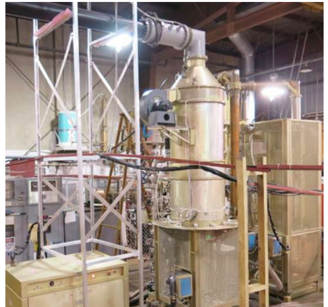
Figure B.2.9 Tetrode based system under factory tests
