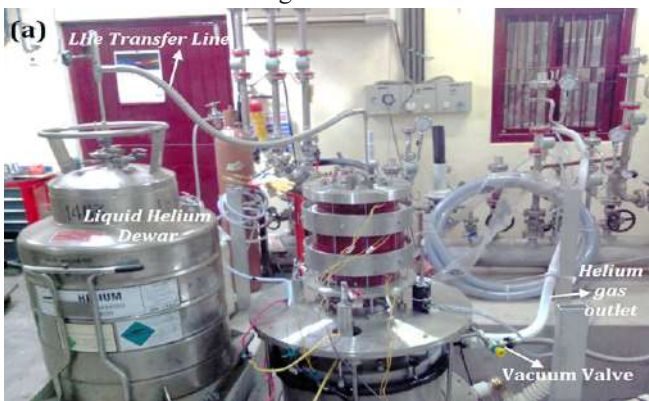
Figure A.2.3 Test set up for 1.65 T Gyrotron Magnet
