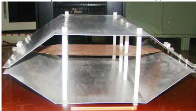
Figure A.3.4.2 The TEM cell developed for calibration of high frequency diagnostics
